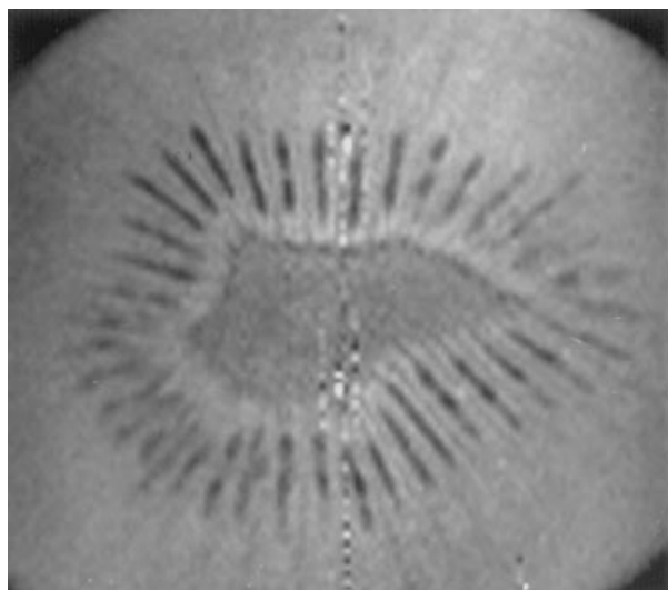
Figure 7. One slice from 16 slices of a kiwi fruit obtained with a RARE sequence 2000/100/90° ( T_2 weighted). Resolution, 0.35 \times 0.35 mm per pixel; thickness, 5 mm; FOV, 44.8 mm; total acquisition time (16 slices), 6 min 24 s.
